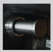
The tensioner can now be fitted to the cylinder head and will fully engage. It should be torqued to the recommended 70Nm.
