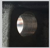
Use an M22 x 1.5mm thread tap to carefully remove any burrs/contamination within the thread of the cylinder head.
